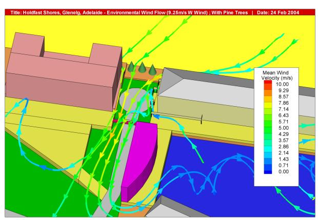
A key aesthetic feature of any proposed 'wind-break' structure to mitigate the problem of wind gusts was that it should have minimal impact upon the surrounding area. Various remedies were assessed in the CFD analysis including the incorporation of vegetation (pine trees), art block sculptures and semi-transparent (wire-mesh) screens.
