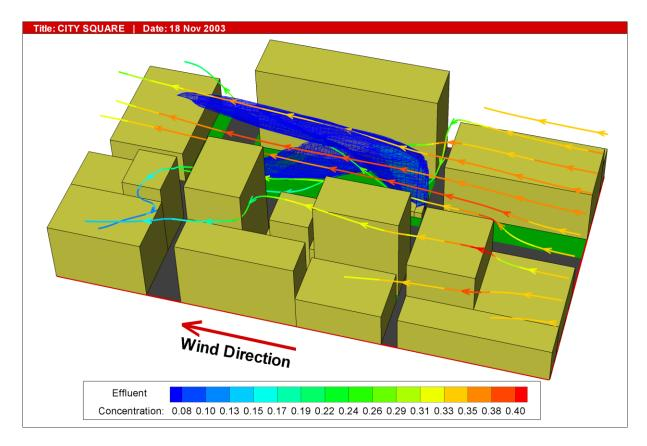
CFD modelling was conducted to assess the effect of stack discharge for different wind conditions. From the results of the analysis, an optimum height and size of duct and exhaust discharge velocity was recommended which would mitigate the effects of the exhaust dispersion upon the café patrons and hotel occupants.
