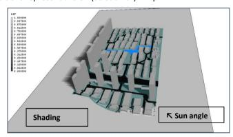
In this example, the ground surrounding the buildings, road, grass and river all have a Z depth of 2m. The ground temperature of 9°C is applied at the lower face of the ground. This represents the constant earth temperature underground.
